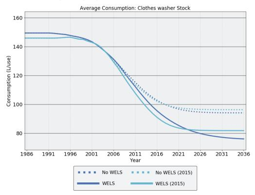
Figure 26 Comparison of average clothes washer water use per load
