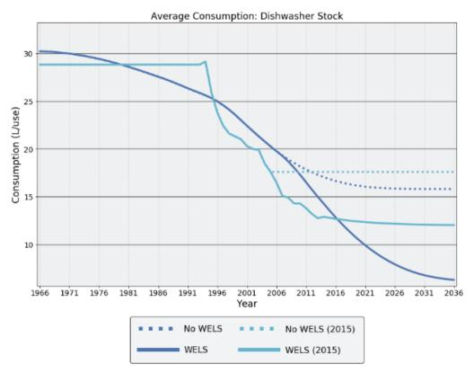
Figure D2 Average dishwasher water use per load comparison
