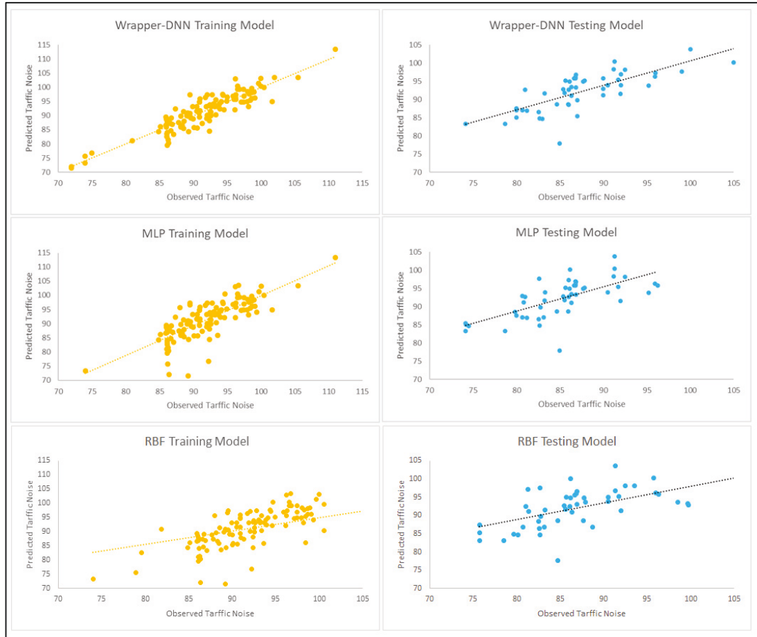
Figure 4.23 Correlation between observed and predicted vehicular traffic noise of WFS-DNN, ANN MLP and ANN RBF models for training and testing.
