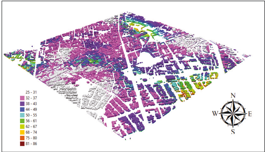
Figure 4.11 Shows 3D average noise prediction map for building at the study area from the 3D noise model.
