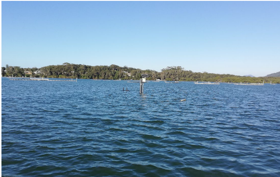
Figure A2 Seabird MicroCAT high accuracy conductivity, temperature and depth (CTD) field sensor deployed in Camden Haven River.
