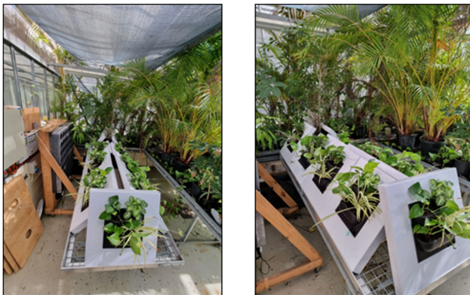
Fig. 1 Experimental small-scale green wall biofilters ( n = 9 ) maintained within a climate-controlled research glasshouse
