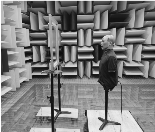
FIG. 2. (color online) Experimental setup using the KEMAR Head and Torso simulator at the listener location with a distance of 70 cm from the panel.
