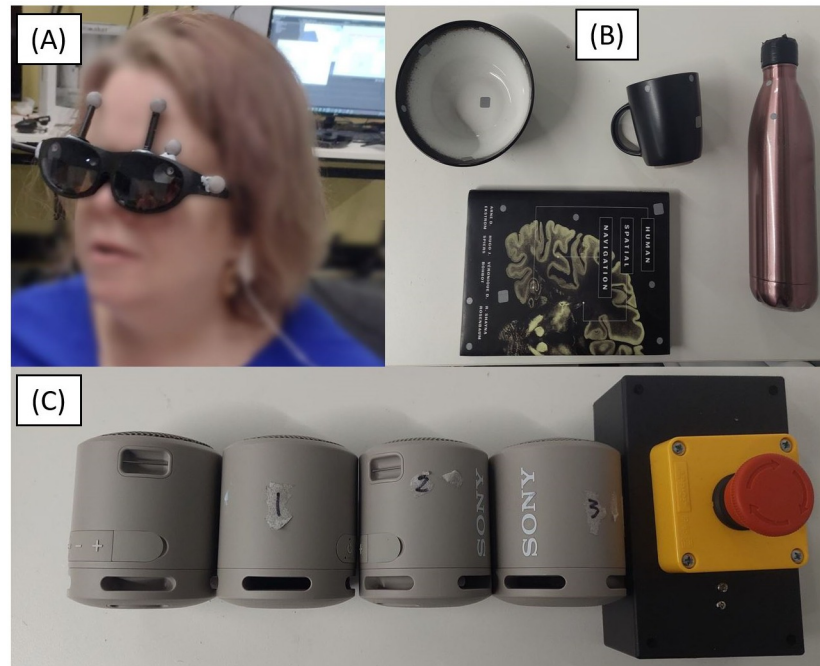
Fig 2. (A) The NReal AR glasses worn by a participant. The grey spheres are the reflective markers that tracked the participant's head movement through motion capture. The participant's face has been blurred for privacy. (B) The household items used during the study. The items (from left to right) are the bowl, book, cup, and bottle. (C) The Sony XB13 Bluetooth speakers and the user response button were used during the study.
