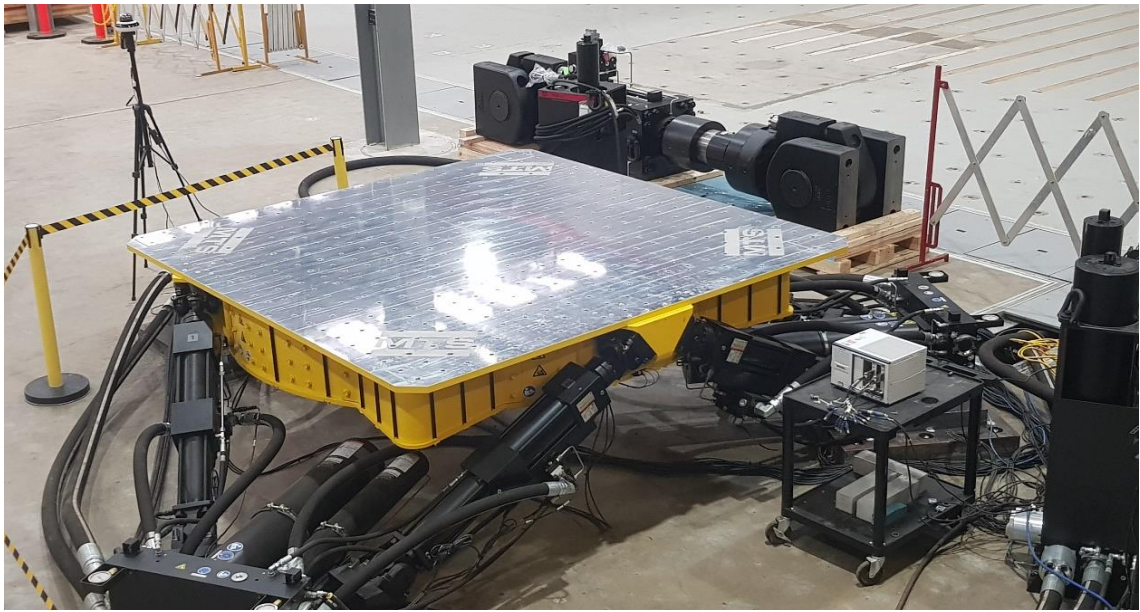
Figure 3.1 Multi-axial seismic simulator at the UTS structural testing facility
