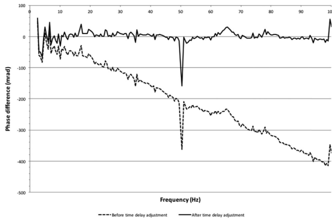
FIGURE 4.2: One of five phase difference plots between the integrated accelerometer and LDV signals used to estimate the phase delay [38]. © 2017 Elsevier, reprinted with permission.
