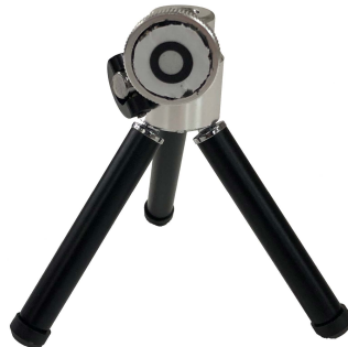
FIGURE A.3: Photograph of the retro-reflective calibration target used during the reference frame alignment procedure.
