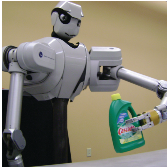
FIGURE 6.6: Photograph of the humanoid robot used in existing acoustic object recognition work [49]. © 2011 SAGE Publications, reprinted with permission.
