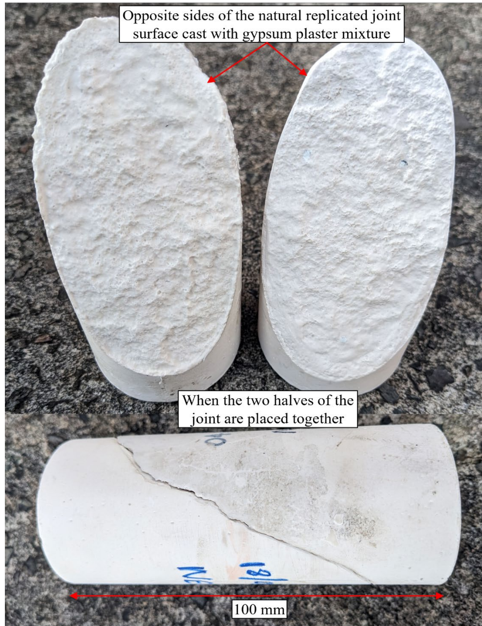
Figure 5.1. (a) The cylindrical hollow mould and rubber moulds of the two opposite sides of the natural replicated joint surface; and (b) The two opposite surfaces of a cast jointed rock specimen.
