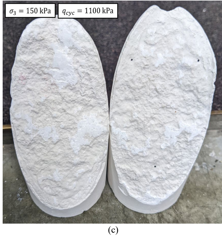
Figure 4.16. Samples of damaged surfaces of the jointed rock specimens at peak deviatoric stress amplitude at confining pressures ( \sigma_3 ) of: (a) 25 kPa; (b) 90 kPa; and (c) 150 kPa.
