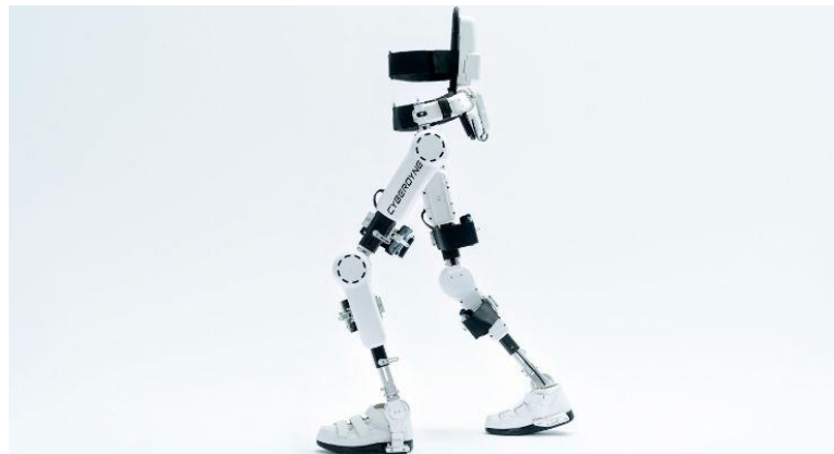
Figure 2.2. Hybrid Assistive Leg 3 rehabilitation device for lower limb spinal cord injuries (Roboticsbiz 2020)
