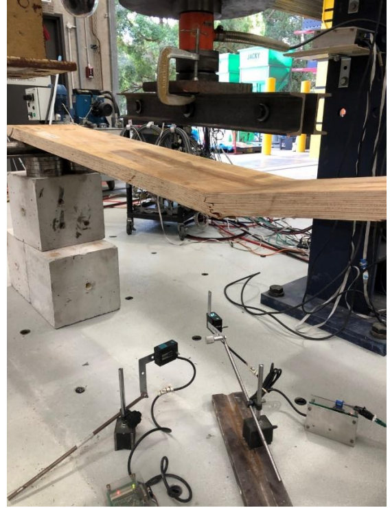
Figure 3.9: Typical bending failure on tensile face of plywood panel
