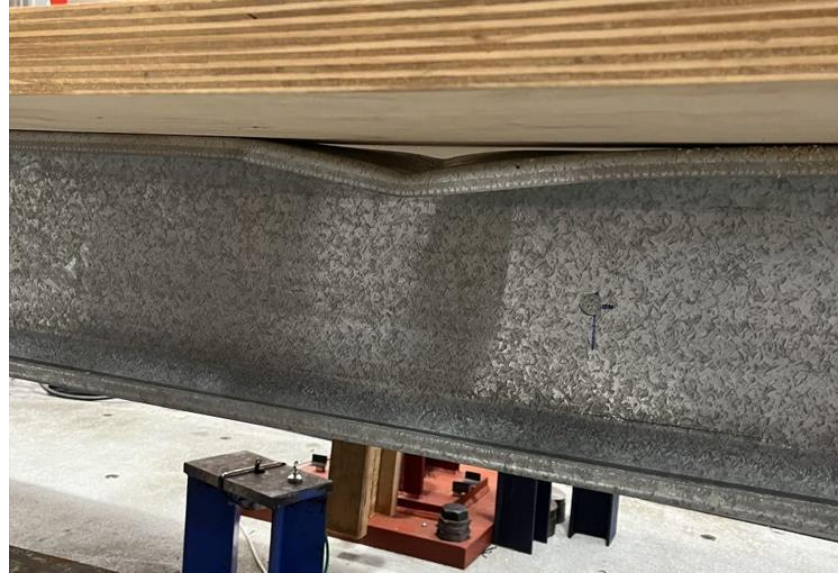
Figure 4.7: Distortional buckling between fixings in the constant moment span (Specimen SP-11)
