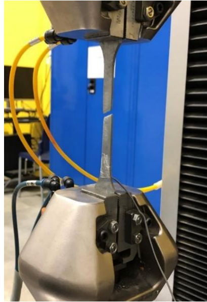
Figure 3.5: Failure of CFS coupon during tensile testing
