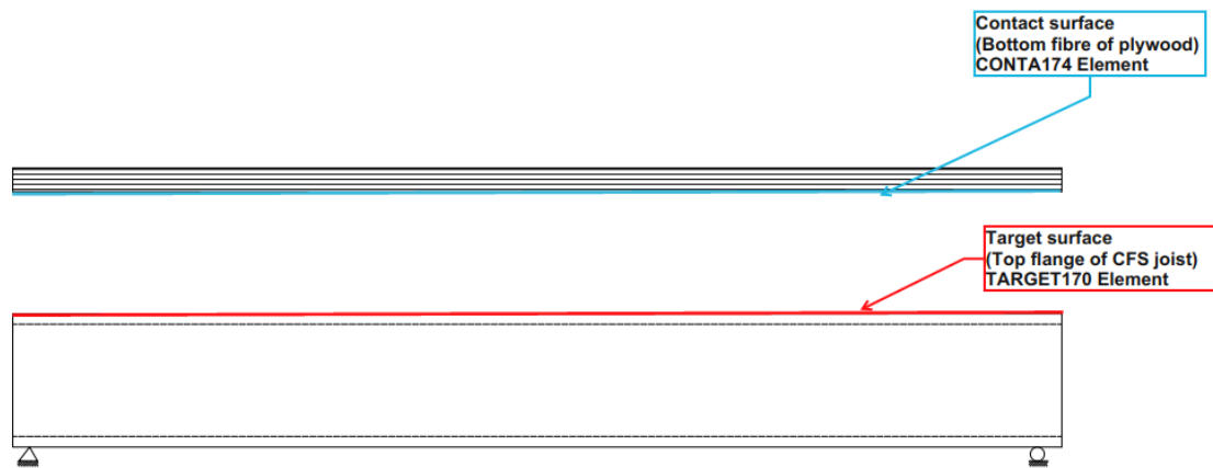
Figure 5.6: Schematic diagram of CFST beam showing contact and target surface for FEM
