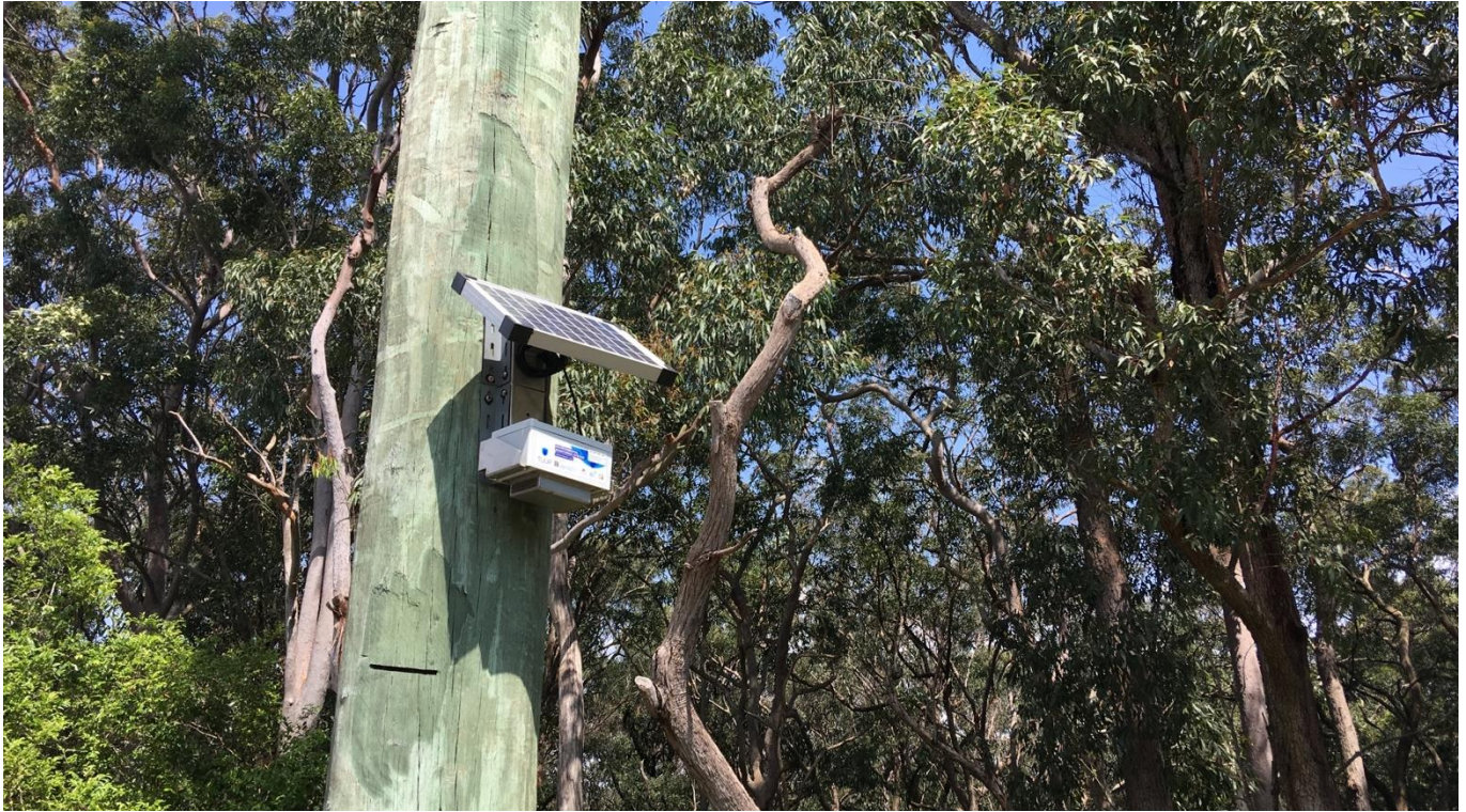
A smart air quality sensing device deployed next to urban bushland in Lake Macquarie, NSW. Image source: UTS
