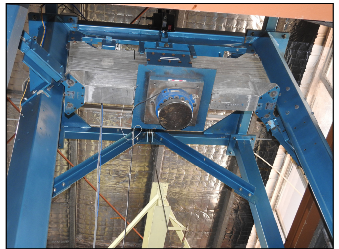
Load cell attached to drop hammer
