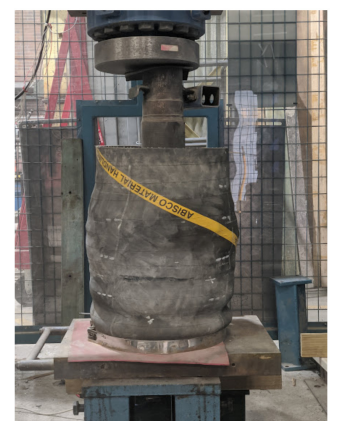
Specimen in contact with drop hammer during the test
