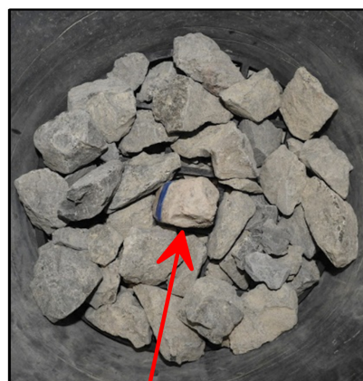
Smart Ballast placed over the rubber grid
