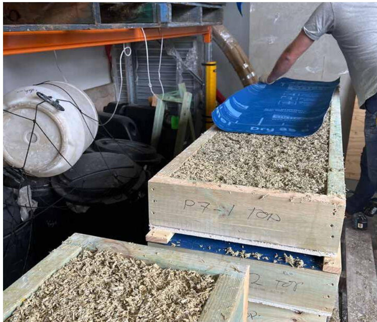
Scaled-down hempcrete structure built at UTS Tech Lab for air quality and thermal performance monitoring. This structure is the first of four to be built
