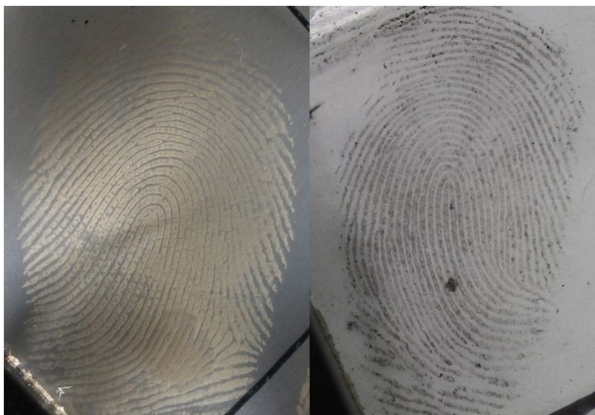
Figure 4 Fingermarks developed on plastic using Fisher/TX (left) with oblique lighting to increase contrast and Sigma/T4 (right) without additional lighting. Shows difference in colour of treated marks
