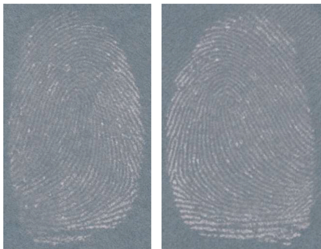
Fig. 3. Two artificial fingerprints detected with VMD_{Au/Zn} on paper.
