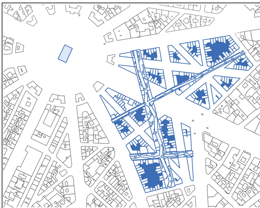
Fig. 20 Final morphology in plan view, showing the skyway intersecting the superblock, and the individual block morphology being contextualised to the surrounding urban fabric
