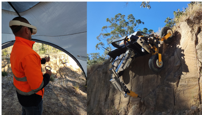
Figure 1: An operator performing rock scaling remotely in VR with HALO.
