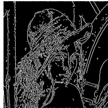
Figure 4: Final edge map of ‘Lena’ obtained from multi-scale edge detection with bilateral filtering.
