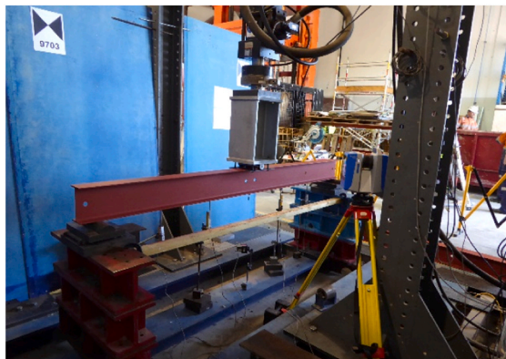
Fig. 5. Layout of TLS and test setup.
