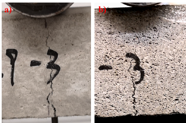
Fig. 9. Examples of the samples' crack in flexural test at 0.8 mm displacement: a) 1700-6-19-0.9 and b) 800-6-19-0.3.
