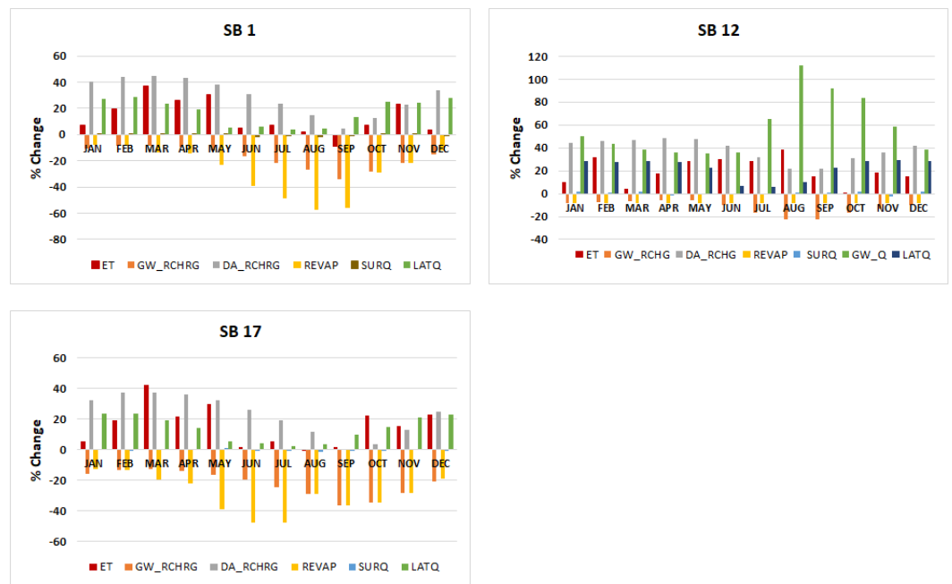
Figure 7. Percentage change in WBCs for sub-basins 1, 17, and 12—comparison between scenario 1 and scenario 2 with change in LULC.
