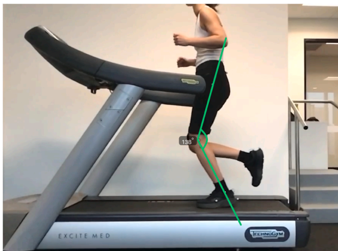
Fig. 7b. Knee Flexion – Mid-stance; Angle between femur (greater trochanter and lateral femoral condyle markers) and tibia (fibular head and lateral malleolus markers).
