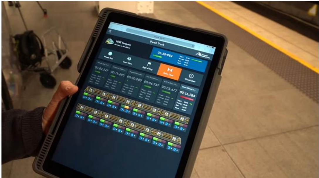
FIGURE 5.11: Tablet application developed at UTS Rapido and used by Fast Track teams at Wynyard station to support dwell time management operations
