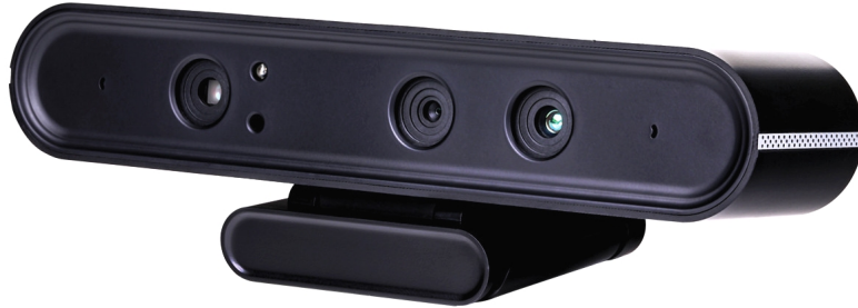
FIGURE 5.1: Orbbec Astra depth-camera used in the Dwell Track system
