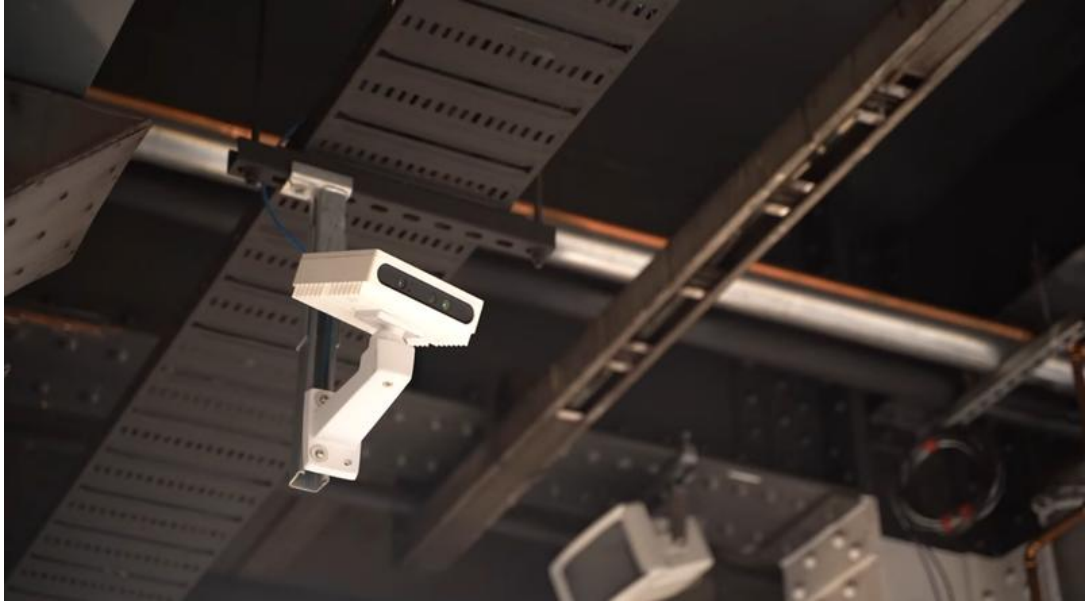
FIGURE 5.10: One of 16 Dwell Track devices installed at Wynyard station as part of a 2019 trial undertaken by Sydney Trains
