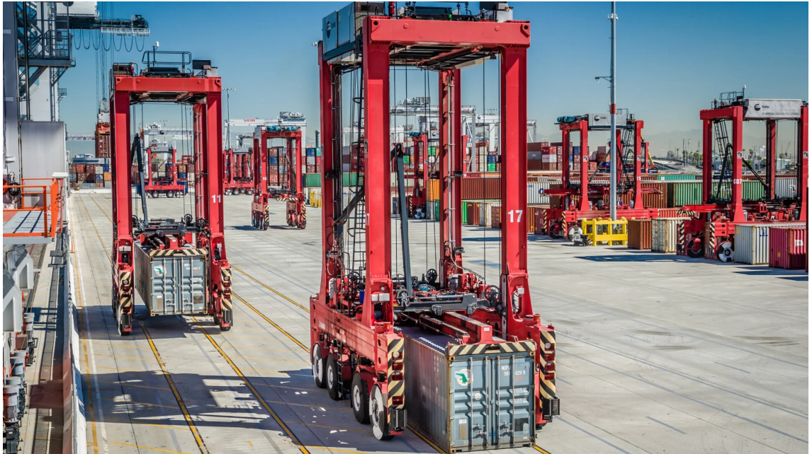
FIGURE 1.1: The Kalmar Autostrad autonomously moves shipping containers around a shipping terminal devoid of humans
