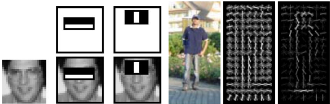
(A) A figure from [12] illustrating the top two features selected by AdaBoost for detecting the face (top row), overlaid on a typical face (bottom row) where they align with the contrast between the eyes and cheeks, and the eyes and nose respectively.
