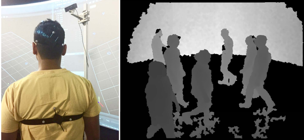
FIGURE 3.3: Left : The sensor platform was mounted on a fixed pole aimed at the centre of the room and the movement of all participants was tracked using optical motion capture with infrared marker cards. Right : A sample depth image taken from the Passing sequence.
