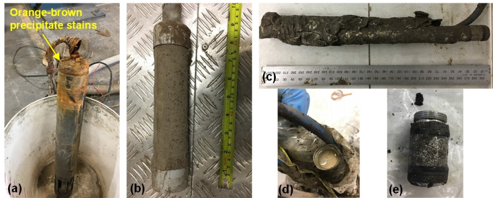
Figure 2: Malfunctioned instrumentation extracted from field sites located in acid sulfate soils: (a) Multi-parameter sensor from Shoalhaven floodplain; (b) Standpipe filter tip from Shoalhaven floodplain; (c) Vibrating wire piezometer from Ballina, NSW and its (d) mineral precipitation on sensor surface and (e) filter tip
