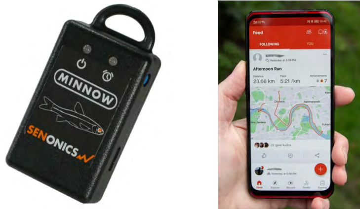
Figure 25 Minnow Sensor 1.0 is used for temperature and humidity data (left), and the Strava application (right) tracks geo-location in real-time during on-field investigations.
