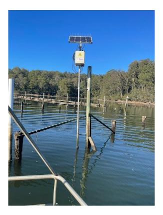
Figure A2 Example of a Seabird MicroCAT high accuracy conductivity, temperature and depth (CTD) field sensor deployed in NSW estuaries.
