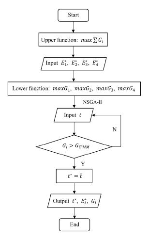
Figure A1. Bi-level multi-objective optimization model algorithm flow.
