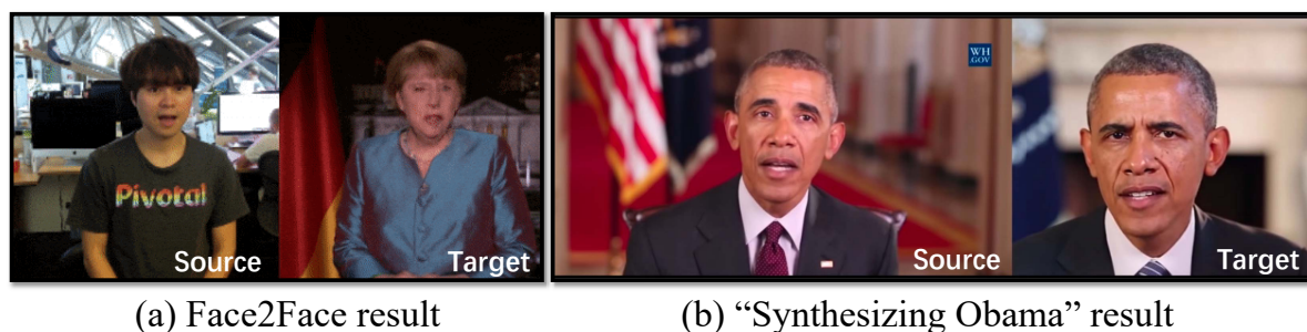
Figure 1.1: (a) The Face2Face result. The source person's facial expression is modified in accordance with the target person's facial expression, which is called facial expression reenactment. Image credit to [139]. (b) The "Synthesizing Obama" result. Given an input Obama audio and a reference video, the system can synthesize photorealistic, lip-synced video of Obama speaking those words. Image credit to [131].
