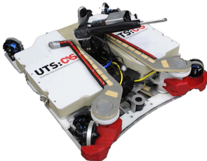
FIGURE 1.2: The submersible pile inspection robot version 3 (SPIR3) ROV.
