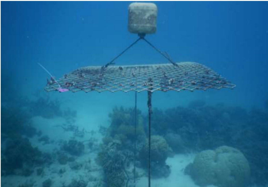
Figure S2.5. In situ floating nursery frame. Nursery frame consisting of 2.0 \times 1.2 m aluminium diamond-mesh, held in place with 2 \times 9 kg Besser blocks and a 20 L float approximately 2 m above the sand at study site 'Rayban' on the Northern Great Barrier Reef.
