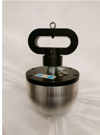
Figure 2: The HIC impact test meter used in this research.
