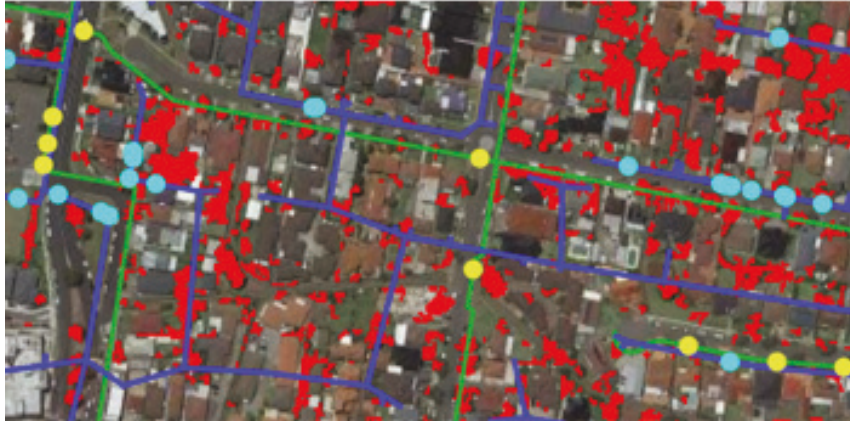
Figure 5.2 An example of our data shown on the map. It includes water pipes (green lines) and failures (yellow dots), sewer pipes (blue line) and failures (light blue dots), as well as tree canopy (red polygons).
