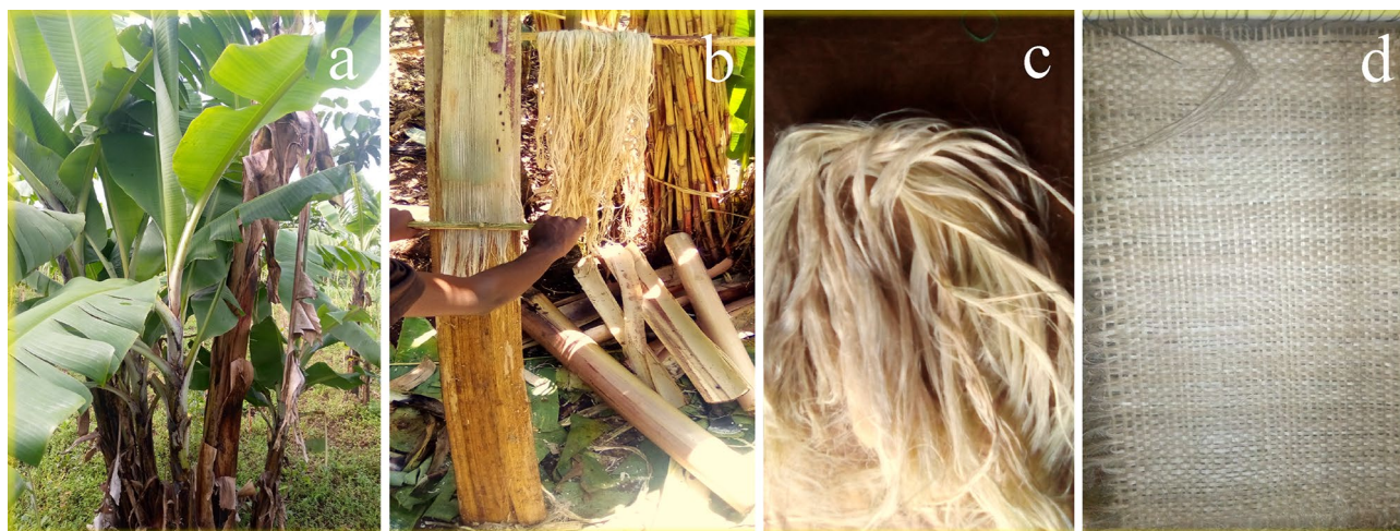
Figure 1. Banana fiber extraction (a) banana plant (b) banana fiber extraction (c) banana fiber (d) banana fiber mat.
