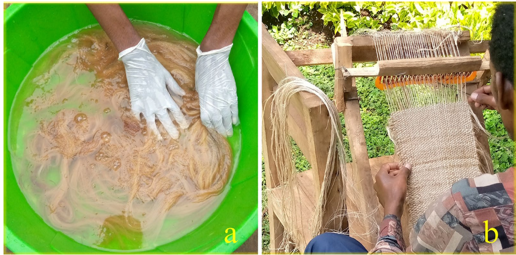
Figure 2. Fabric preparation (a) Treated fiber (b) Fiber mat weaving.
