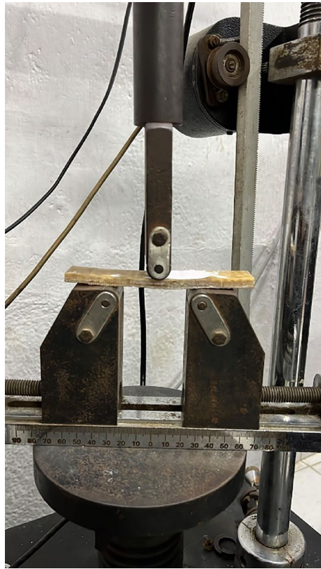
Figure 5. Three-point bending test on banana sandwich composite.
