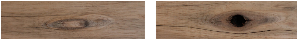
Figure 3.4 Knots in timber boards. Live (left) and dead (right)
