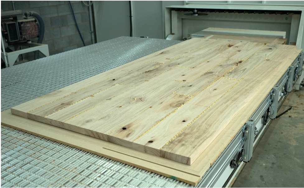
Figure 4.31 Panel positioned in the CD zone of the CNC router
