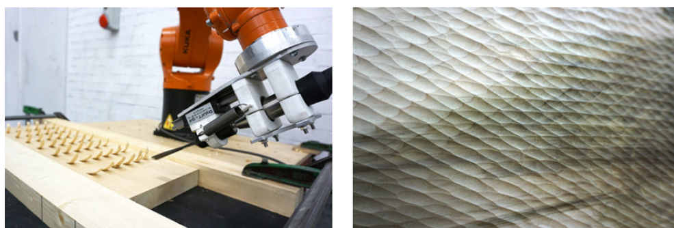
Figure 2.21 Adaptive robotic wood carving with material force feedback (From Brugnaro & Hanna, 2018. Copyright 2018 Springer. Reproduced with permission)
