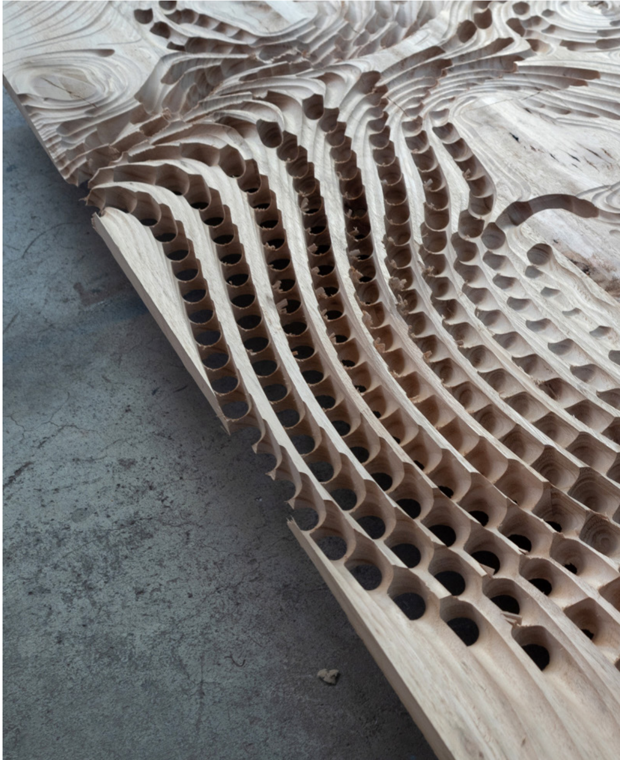
Figure 4.35 Detail of demonstration panel, showing augmentation and perforation of surface
