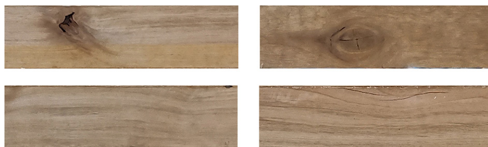
Figure 3.14 Natural timber features: (clockwise from top left) dead knot and colour variation; live knot; grain variation; surface checking
