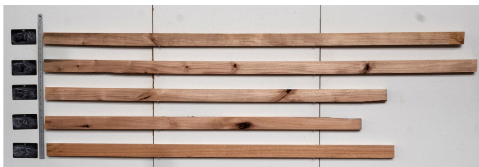
Figure 3.10 Grouping of five timber boards for image high resolution RGB capture
