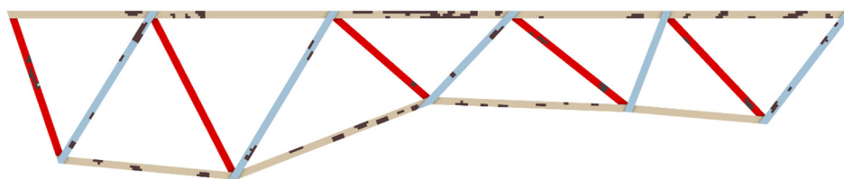
Figure 5.43 Staggering of truss web diagonals to minimise thickness. Blue elements are on front face of top and bottom chords, red elements are positioned at the rear
