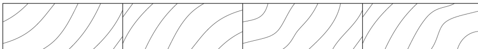
Figure 3.15 End grain of timber boards arranged to oppose the natural cupping force.
