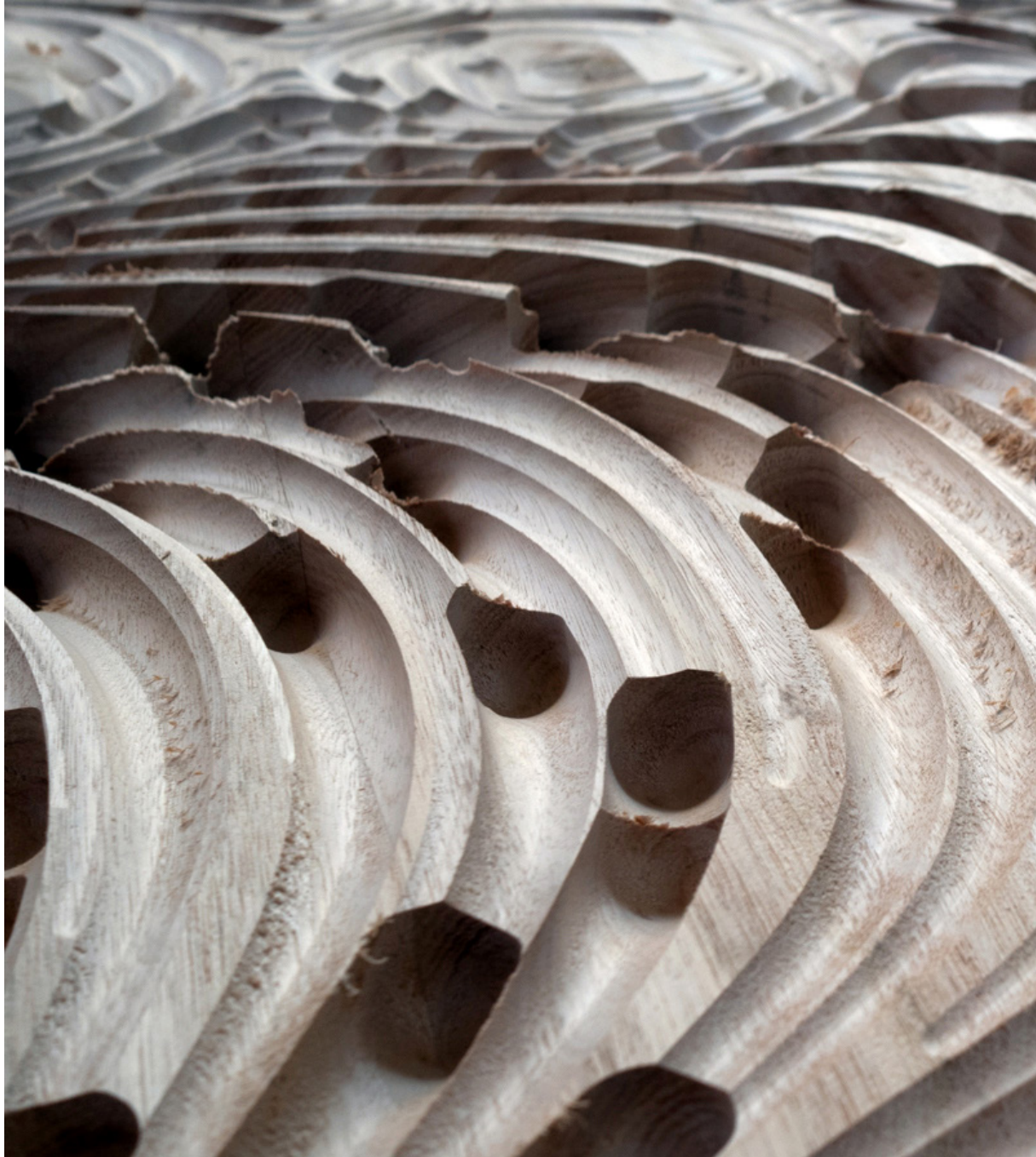
Figure 4.36 Detail of demonstration panel, showing surface augmentation and material tear-out
