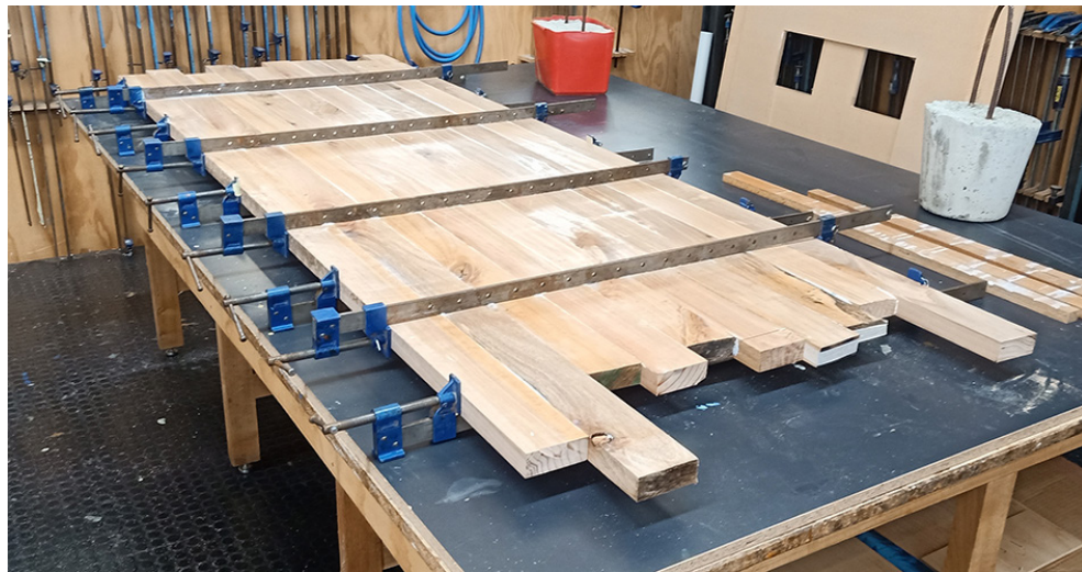
Figure 3.16 Demonstration panel lamination process for Probe 3
