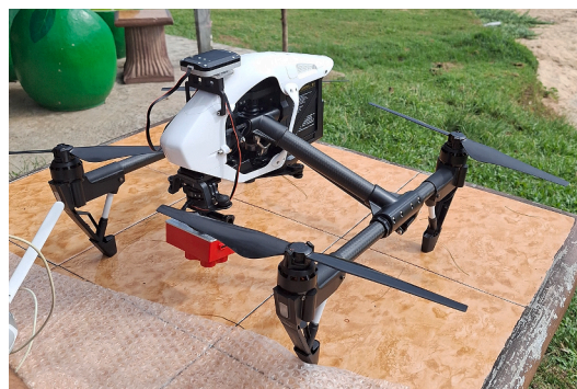
Fig. 4. DJI Inspire 2 equipped with MicaSense RedEdge-M camera sensor.
