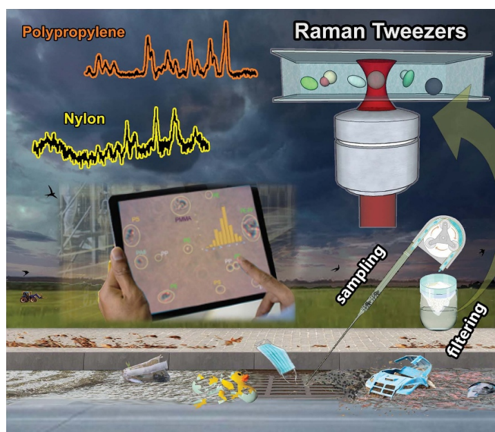
Figure 46. Field-deployable spectroscopic optical tweezers will be designed to be compact and integrated with fluidic circuits capable of extracting samples from the environment, and filtrate and concentrate particles, prior to multispectroscopic analysis for plastic particle classification by size and materials.
