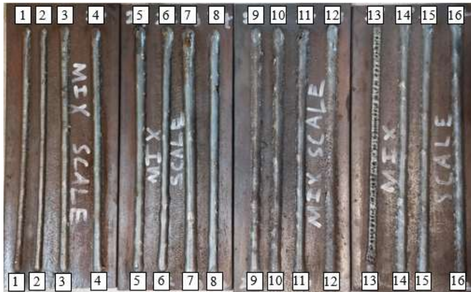
Figure 6.3 - Weld Bead Profiles
