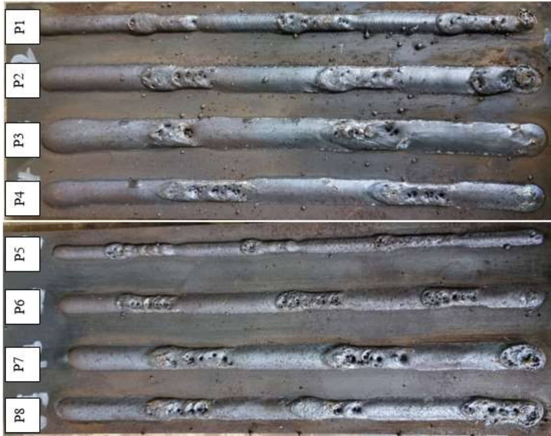
Figure 5.9 - Porosity Test Plates
