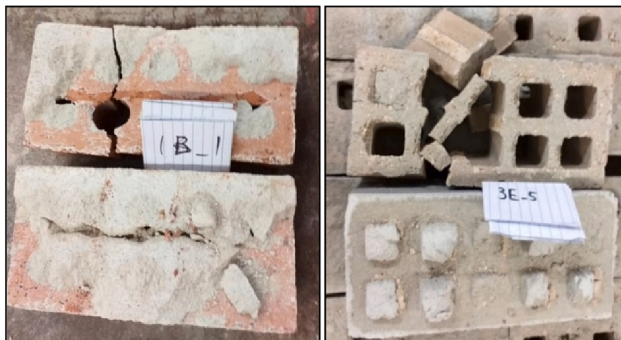
Fig. 9. Examples of unit splitting during or after testing due to over-tensioning of bolts.
