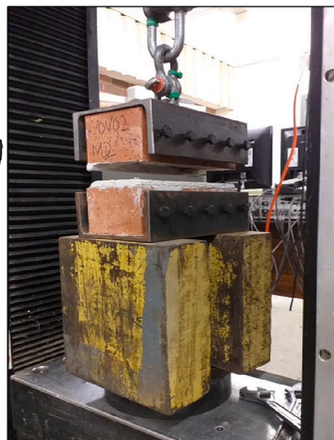
Fig. 8. Isometric and as-constructed image of apparatus for direct tension on unit-mortar interface; image captured after failure of joint.
