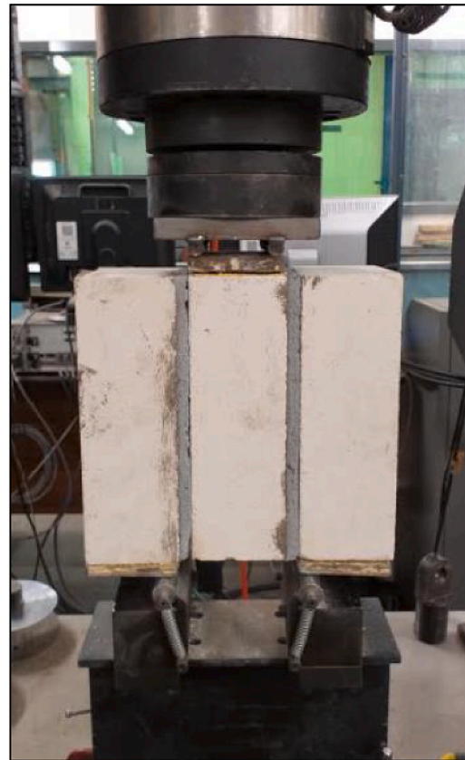
Fig. 6. Schematic diagram and test set-up of the triplet shear test. Adapted from EN1052-3 [7].
