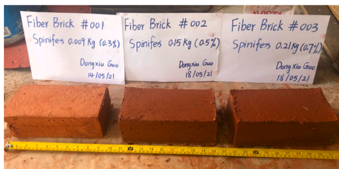
Fig. 2. Mudbrick reinforced by Spinifex fibre which is wildly used by Indigenous people in tool making.
