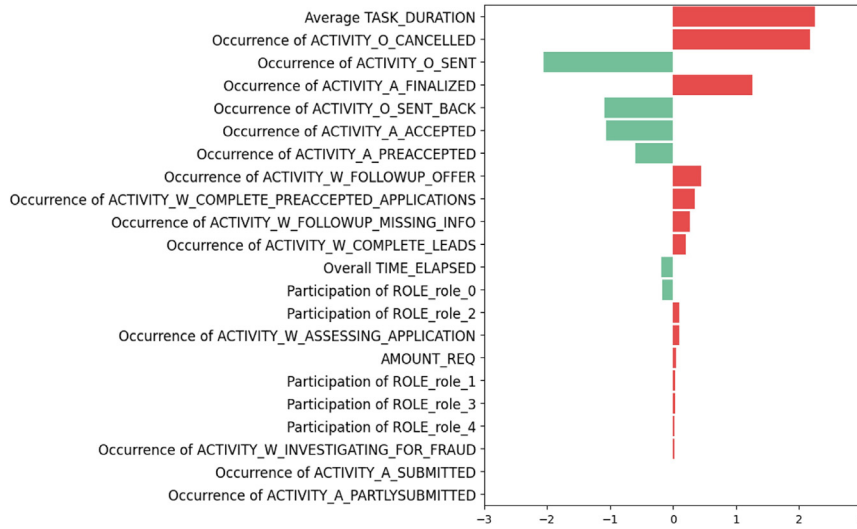
Fig. 20. Global explanation generated by logistic regression model identifies the activity O_CANCELLED and high Average TASK_DURATION to be the top features that influence the decision of A_UNSUCCESSFUL.
