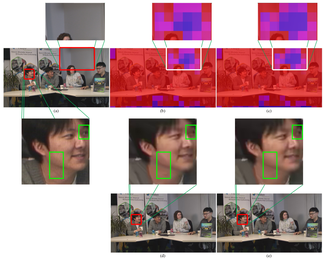
Figure 7. Bit heatmaps and reconstructed frame of intra coding at 384 kbps: (a) original frame, (b,d) RC-HEVC, and (c,e) proposed method.
