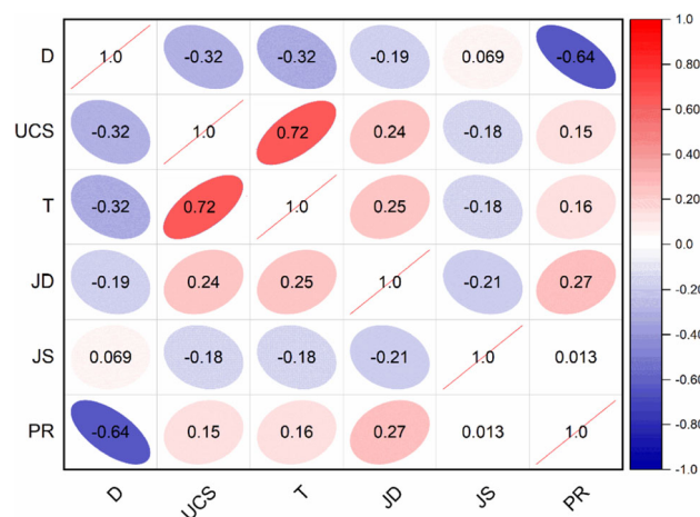
Fig. 4 An overview of the correlation matrix for all data samples (inputs and output)
