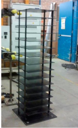
Figure 8. Completed fixed-base model of shaking table tests (Tabatabaiefar and Mansoury, 2016; Zhang and Far, 2022).
