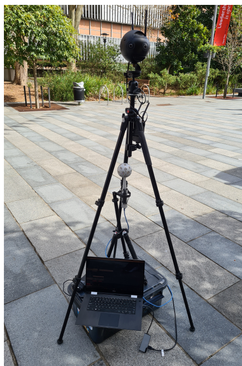
Figure 2. The camera and microphone setup used for capturing 360-degree video and spatial audio, illustrating the equipment configuration and arrangement for creating immersive virtual environments used in Virtual Urban Field Studies.
