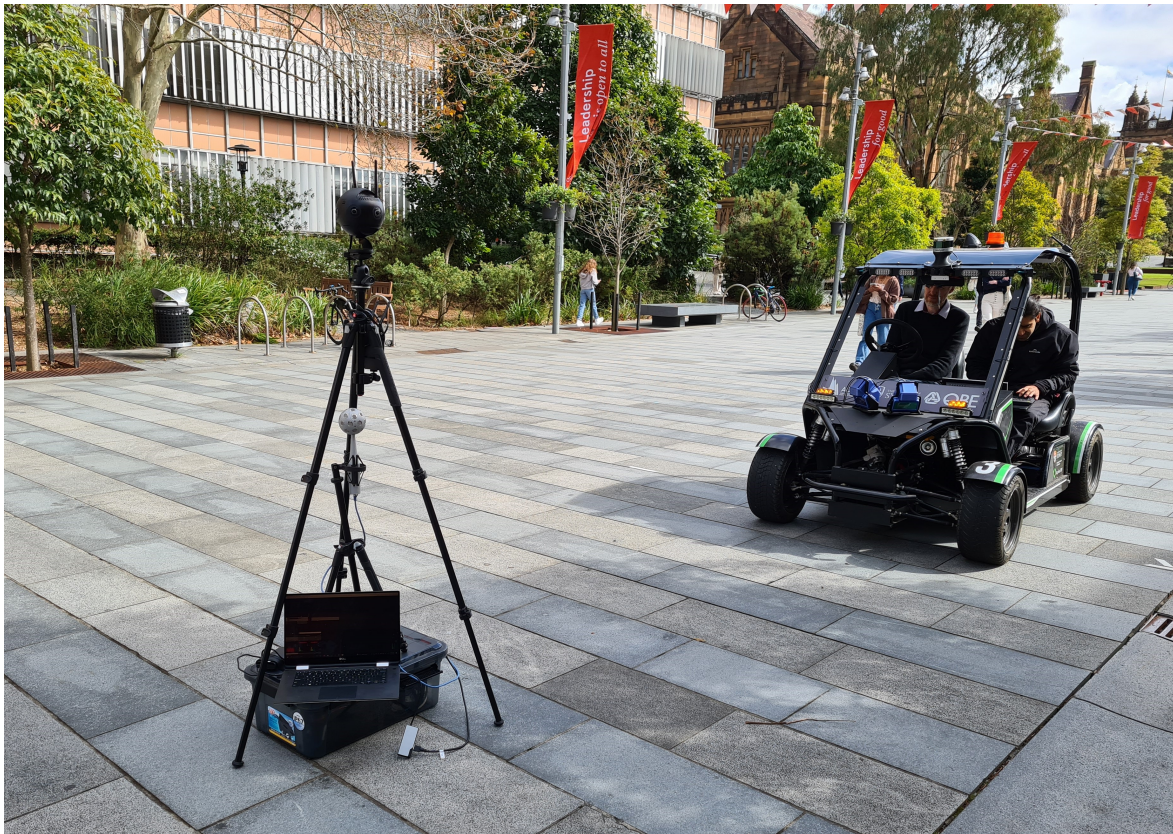
Figure 1. The autonomous vehicle during technical testing, having navigated through a shared space and come to a stop. The scenario is being recorded by a 360-degree video camera and spatial microphone to create an immersive virtual environment for a Virtual Urban Field Study.
