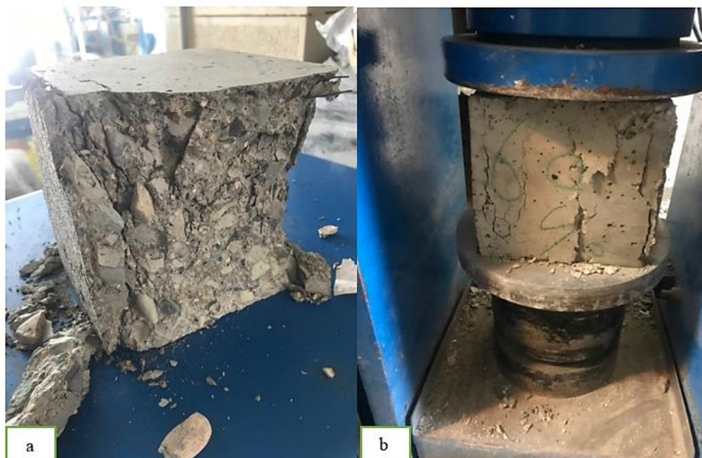
Figure 7. (a) Compressive failure mode; (b) secondary compressive failure mode.
