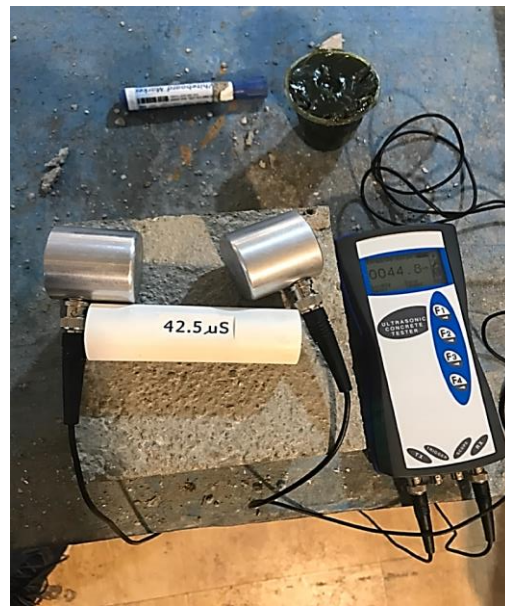
Figure 3. A view of the ultrasonic concrete tester.
