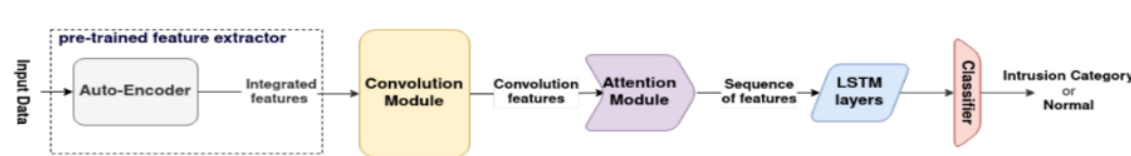
Figure 4.4 : An overview of the proposed method for an IDS
