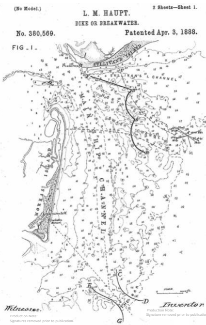
Figure 7: US 380569 "Dike Or Breakwater" popularly known as the Reaction Breakwater which excavates channels and stabilizes shorelines through the controlled forces of water. (Source: European Patent Office, https://www.epo.org/en )
