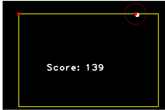
FIGURE 5.1: The experimental task requires participants to follow the red target dot with the white dot while remaining within the red circular boundary. The task becomes more intense as the radius of the boundary reduces with time. A Score is calculated based on the time that the participant could stay within the boundary. It increases if the participant is able to remain within the boundary. Otherwise, it reduces.
