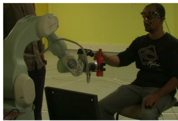
(b) Example of Cooperative Interaction: human and robot hand-over a bottle. [49]
