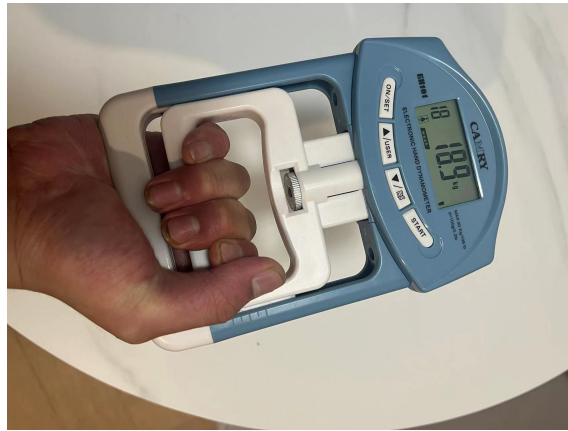
FIGURE 6.6: Hand Dynamometer used for measuring maximum isometric force.
