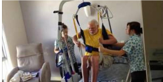
FIGURE 1.5: ‘Smart Hoist’: a patient lifting device equipped with sensors and powered wheels. Although functioning as an advanced patient lifter, it significantly eases the operational effort, potentially reducing lower back injuries among caregivers.
