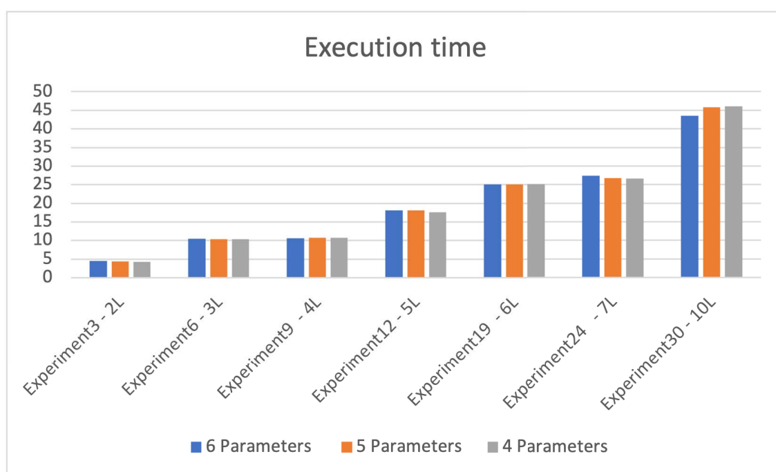
Figure 7.21 : The average execution time of best 7 DNN experiments with a different number of layers and neurons
